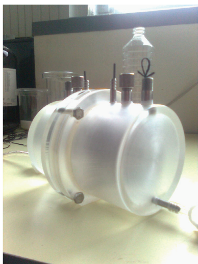
Fig. 2. Picture of the MFC constructed.
