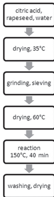
Fig. 2. Scheme of cellulose citrate preparation.
