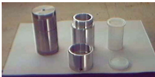
Fig. 1. SS autoclave fabricated for reaction.
