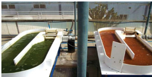
Fig. 2. Cultivation of Dunaliella salina in raceways with SWRO brine [25].
