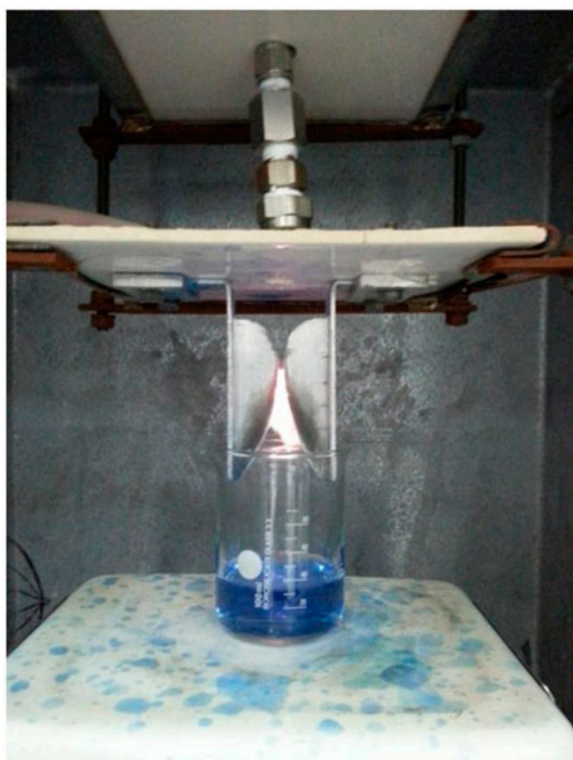
Fig. 3. A photograph of the gliding-arc plasma apparatus.
