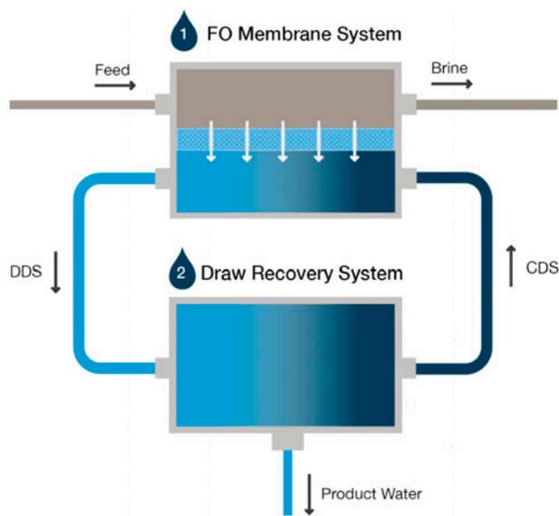
Fig. 1. High level view of a forward osmosis process, which relies on two primary systems: (1) the FO membrane system and (2) the draw recovery system. Notes: CDS: concentrated draw solution and DDS: diluted draw solution.
