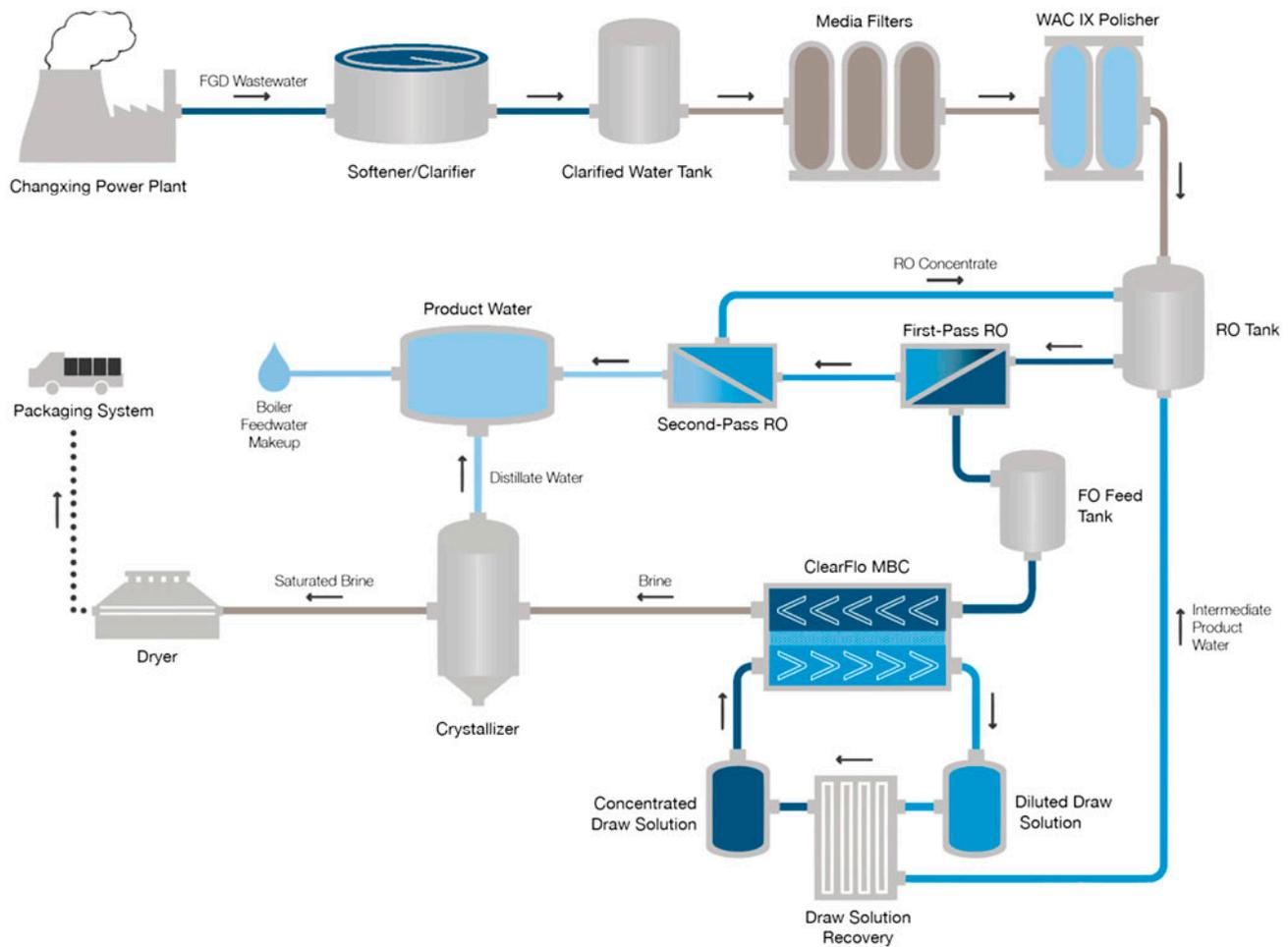
Fig. 5. Process flow schematic of the Changxing Power Plant water treatment, including pretreatment, MBC (i.e. RO, FO, and thermal recovery systems), crystallization, and drying.
