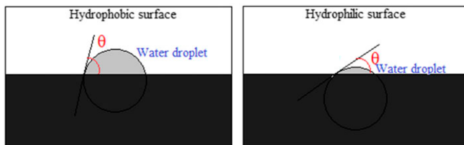
Fig. 4. Contact angle measurement between water droplet and membrane surface (Adapted from [84]).
