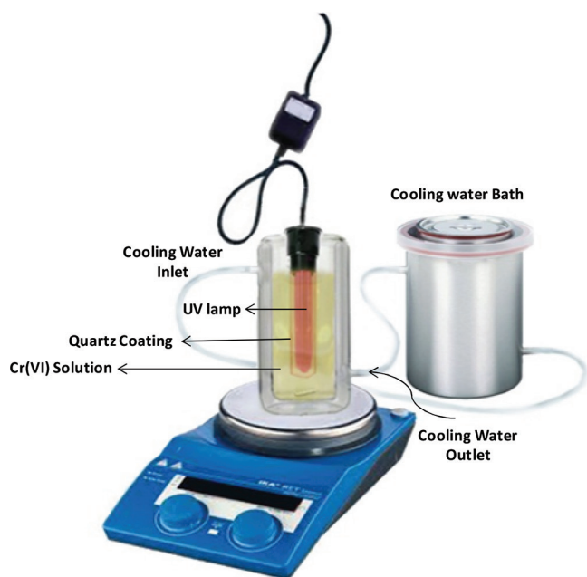
Fig. 2. Experimental set-up for the photocatalytic reduction of hexavalent chromium.
