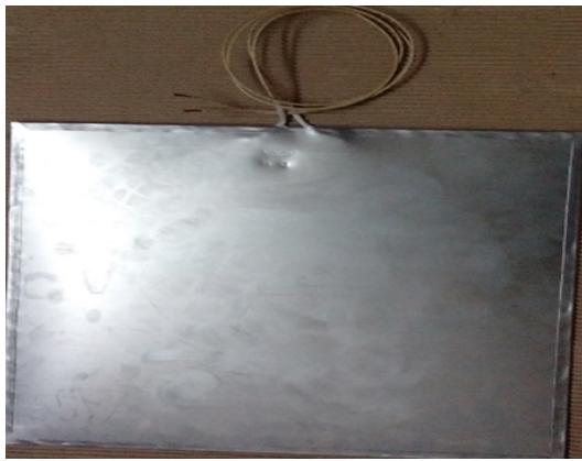
Fig. 3. Actual photograph of electrical heater.
