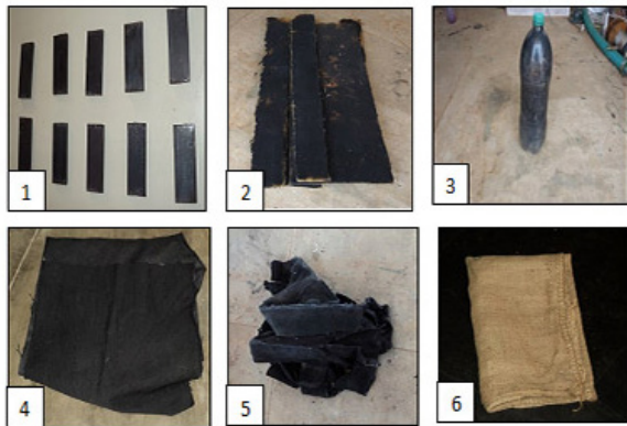
Fig. 7. Photographic view of materials used. Note: 1 – Mild steel pieces; 2 – polystyrene sponge; 3 – lack dye; 4 – black cotton cloth; 5 – waste cotton pieces and 6 – jute cloth.
