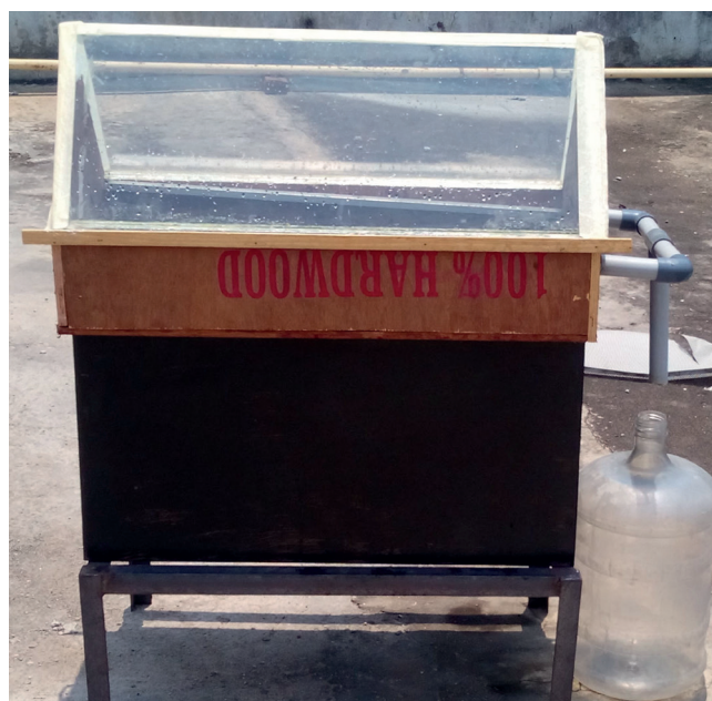
Fig. 2. Double slope solar still without external modifications.
