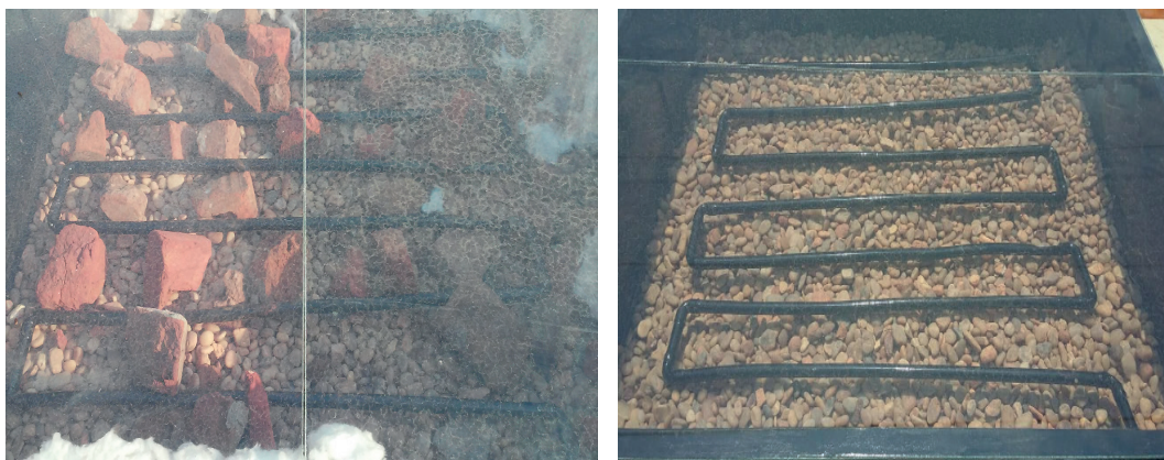
Fig. 1. Internal arrangement of flat plate collector.
