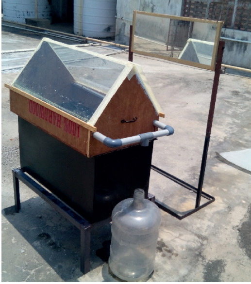
Fig. 4. Double slope solar still with external reflecting mirror.
