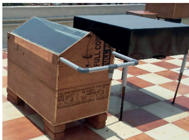
Fig. 3. Double slope solar still with flat plate collector.
