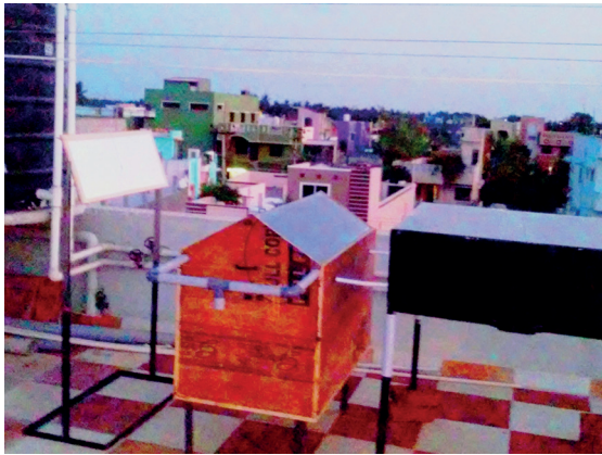
Fig. 5. Double slope solar still with external reflecting mirror and flat plate collector.
