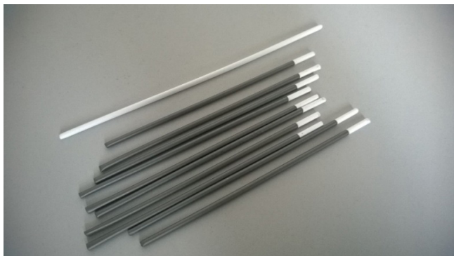
Fig. 9. Membranes made of polypropylene coated with titanium [12].
