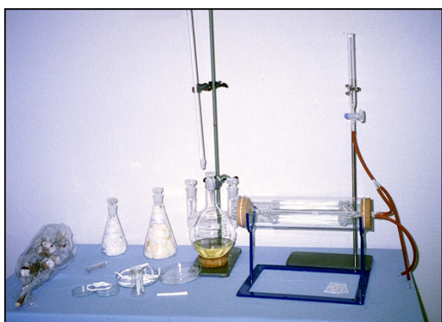
Fig. 2. Prototype of an artificial kidney according to Prof. Abel's idea [1].
