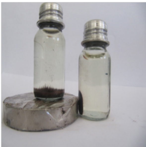
Fig. 3. Demonstration of magnetic separation at 30 s.
