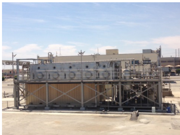
Fig. 3. OT-LT MSF pilot plant in SWCC-DTRI, Jubail, KSA.
