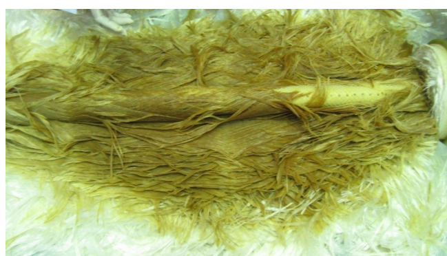
Fig. 5. A view of inner portion of the membrane close to the feed tube showing anthracite particles.
