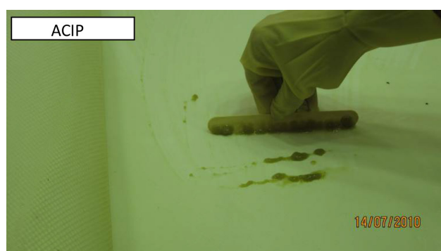
Fig. 15. Foulant being scraped off from the ACIP membrane element.
