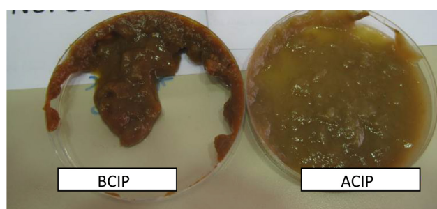
Fig. 16. View of foulant collected from both membranes.
