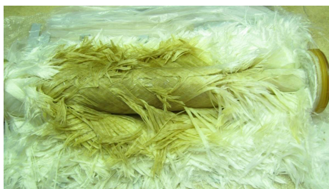
Fig. 3. A view of middle portion of the membrane with discoloration.
