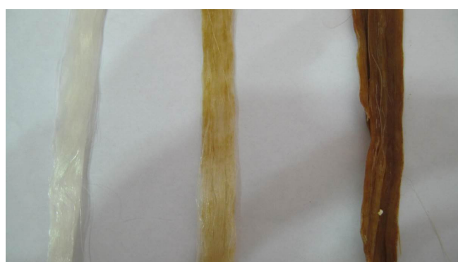
Fig. 6. Distinct color difference among the membrane fibers collected from outer, middle and inner portion of the membrane (from left to right).
