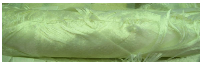
Fig. 2. A closer view of membrane showing very clean outer fibers.
