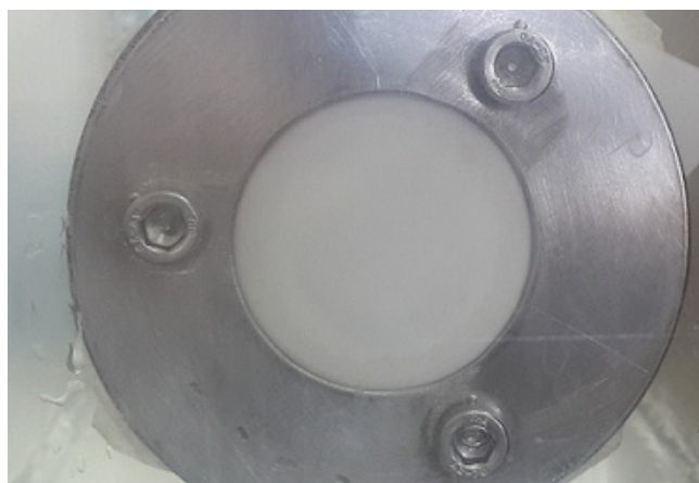
Fig. 2. Flat-sheet membrane and frame configuration.
