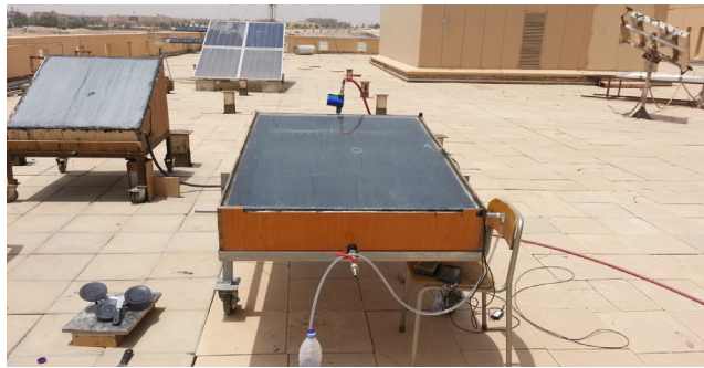
Fig. 2. A pictorial diagram of the inclined solar distillation system (control system - ISWD).
