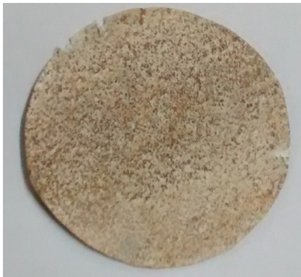
Fig. 2. Silver decorated hybrid M-12 membrane.
