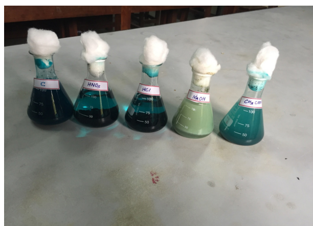
Fig. 14. Desorption study under different desorbing medium.
