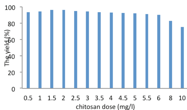
Fig. 7. Effect of chitosan dose on bentonite removal.
