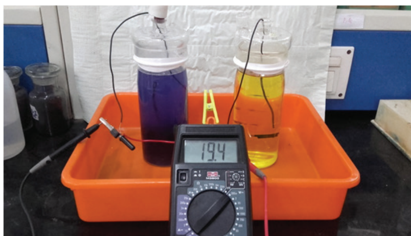
Fig. 1. Schematic and photograph of two-chambered microbial fuel cell with textile dye effluent as the anode substrate.
