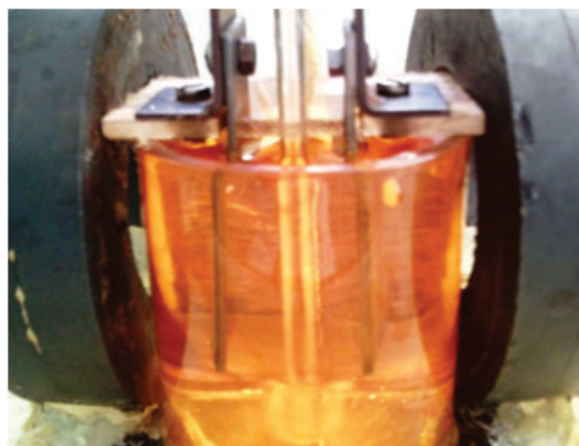
Fig. 1. The apparatus of EC with MF magnets placed for the treatment of MO.
