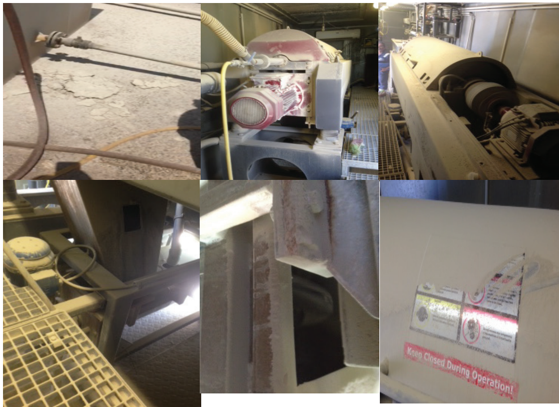
Fig. 7. Fine dust coming out as a discharge from the solid side compartment.
