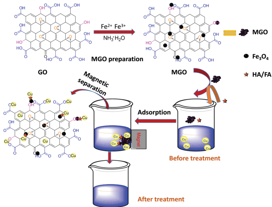
Fig. 8. Schematic illustration for the preparation process of MGO and its application in the removal of Cu(II) from aqueous solution.
