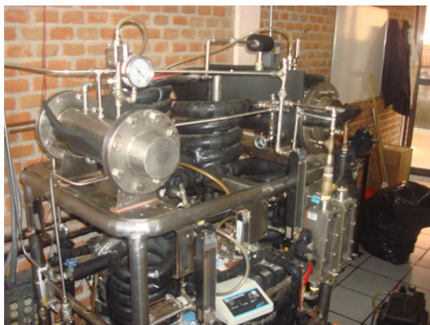
Fig. 1. Experimental absorption heat transformer coupled for water purification.
