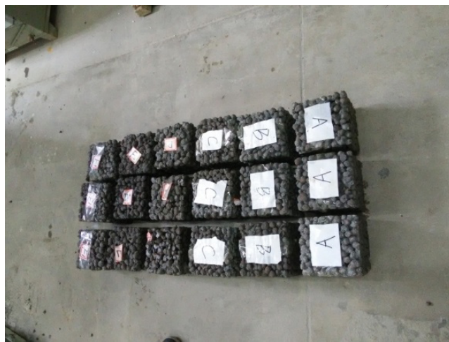
Fig. 1. Porous concrete experiment cubes.
