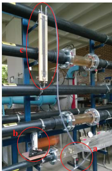
Fig. 3. Configuration for measurement of the pressure loss on MP (a – aerator, b – rotameter and c – differential manometer).
