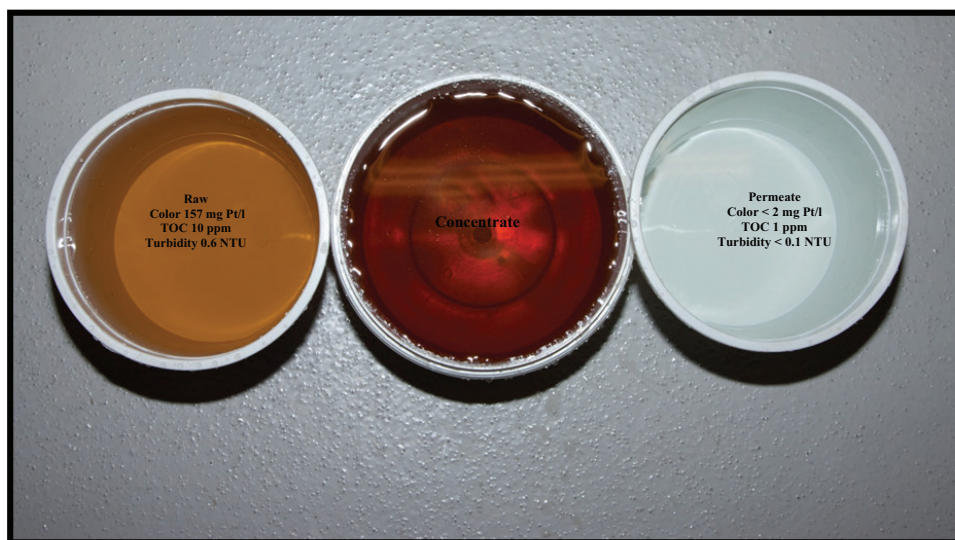
Fig. 6. Water quality comparison of the different streams obtained during the membrane filtration process.
