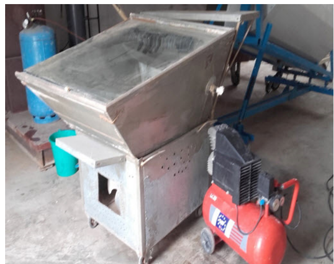
Fig. 2b. Actual photograph of SSDHP with air pump.
