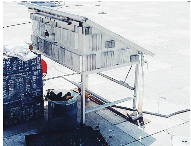
Fig. 6. Fin configuration on the sidewalls of the solar still.
