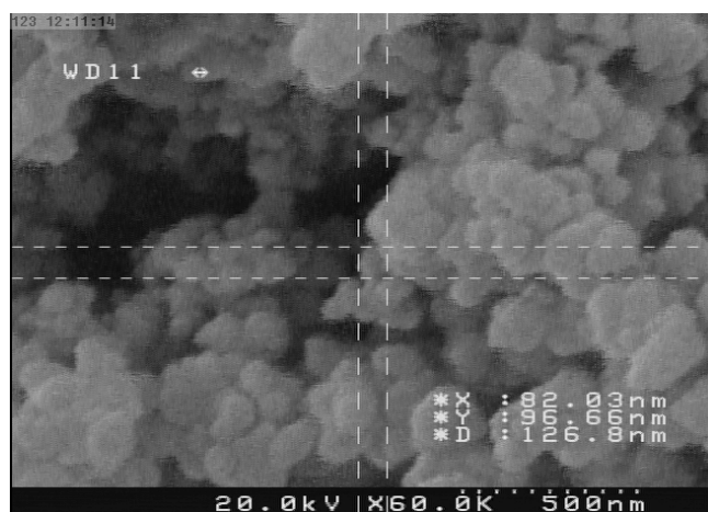
Fig. 2. SEM images of PPY/perlite.
