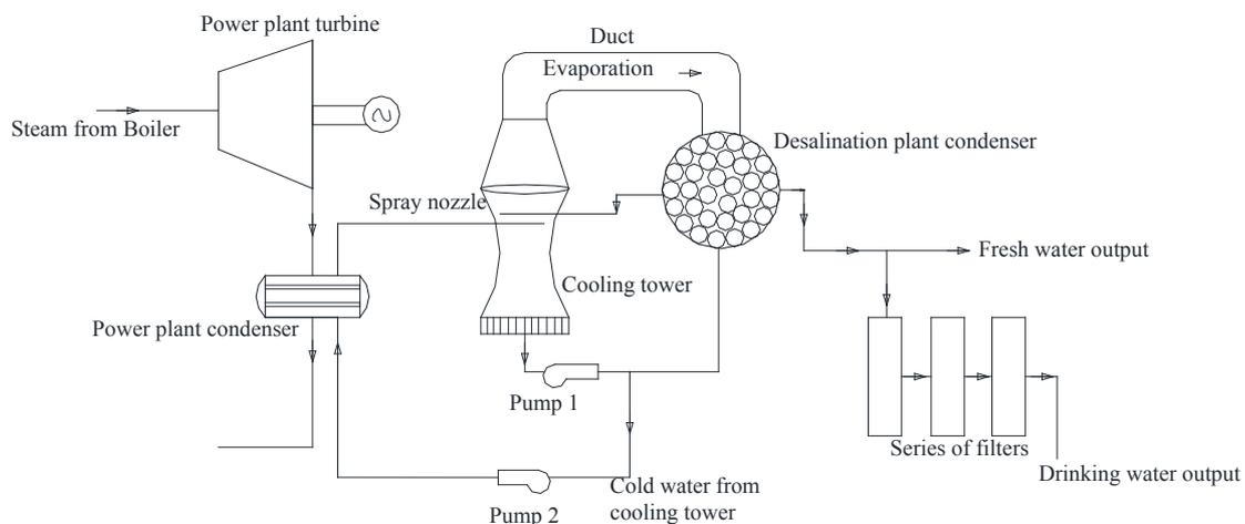
Fig. 1. Schematic diagram of the cooling tower coupled with desalination plant.
