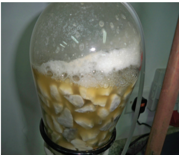
Fig. S1. White stone, the supporting material and the biofilm system formation.
