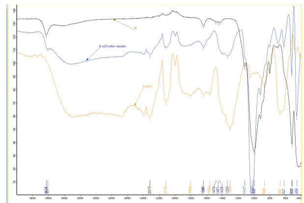
Fig. 5. FTIR spectra of: (a) bentonite; (b) B-nZVI; and (c) B-nZVI after reaction.
