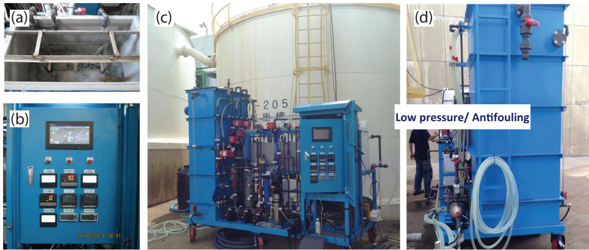
Fig. 2. Photos of the mobile pilot plant on site: (a) top-view of sMF tank, (b) control panel, (c) front-view and (d) side-view of the IMS.
