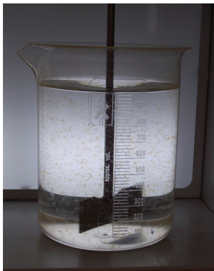
Fig. 2. Creation of flocs after the dosing of water glass, slow mixing stage.
