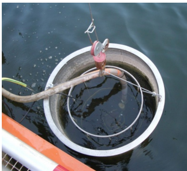
Fig. 5. Catchment point with double filter in the Náquera Research Centre (CIN).
