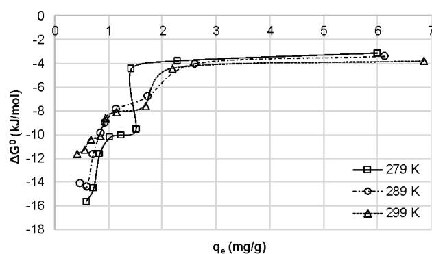
Fig. 4. Gibbs free energy changes dependence on ammonium uptake quantity at different temperatures.
