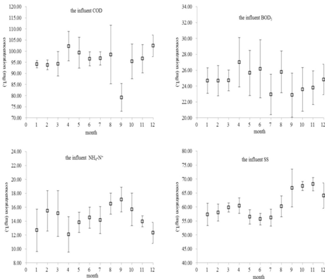
Fig. 1. The fluctuation of influent COD, BOD<sub>5</sub>, NH<sub>4</sub>-N<sup>+</sup> and SS values in LS in 2015.
