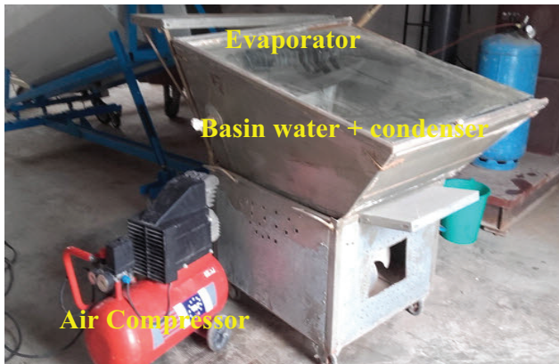
Fig. 1b. Actual photograph of hybrid single slope solar still coupled with an air pump.
