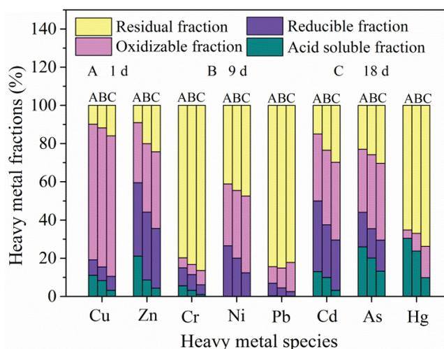
Fig. 7. The variation of heavy metal fractions during biodrying process.
