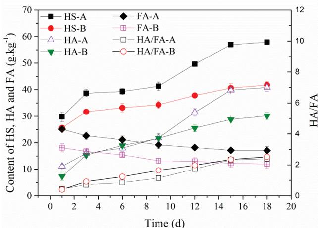
Fig. 5. Variation of humic matter and its composition during biodrying process.
