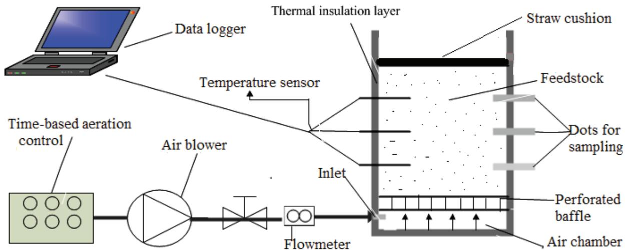
Fig. 1. The schematic diagram of the biodrying system.
