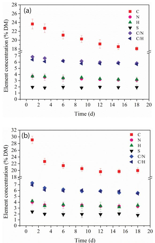
Fig. 6. Element variation during biodrying process: (a) trial A (straw as bulking agent) and (b) trial B (sawdust as bulking agent).
