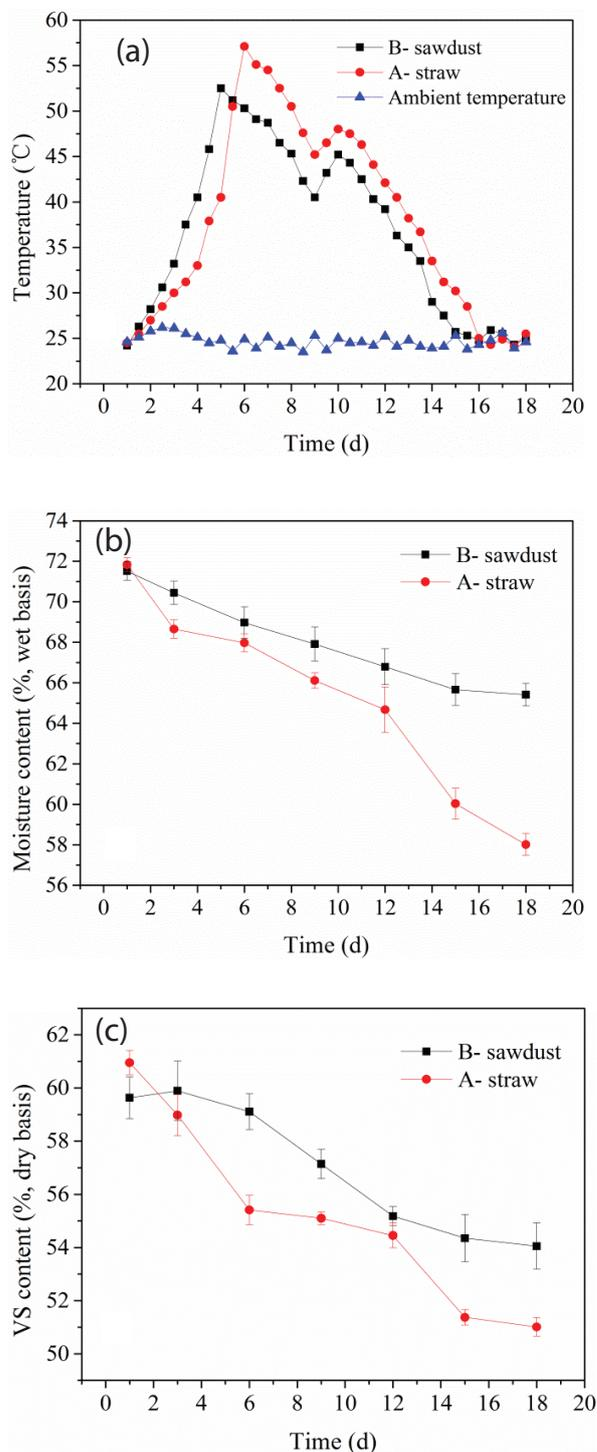
Fig. 2. Performance of the storage sludge biodrying process: (a) mean temperature; (b) moisture content; and (c) VS content.
