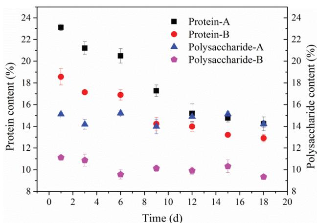
Fig. 4. The variation of protein and polysaccharide during biodrying process.
