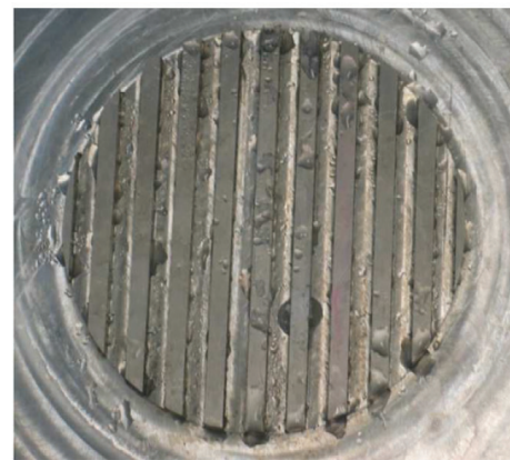
Fig. 6. Channeled coolant plate used for condensation in AGMD [81].
