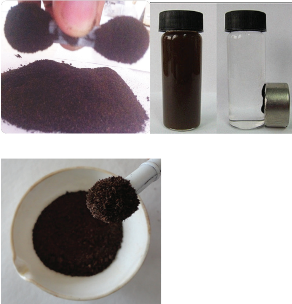
Fig. S1. Checking the magnetic property of \text{Fe}_3\text{O}_4 and \text{Fe}_3\text{O}_4@\text{SiO}_2 particles with magnet.
