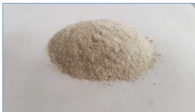
Fig. 2. Crushed struvite recovered from the pipe.
