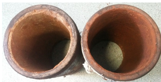
Fig. 1. Two pipe sections with cement coating (left) and without cement coating (right).
