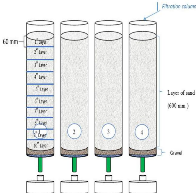
Fig. 3. Schematic of the filtration columns used.
