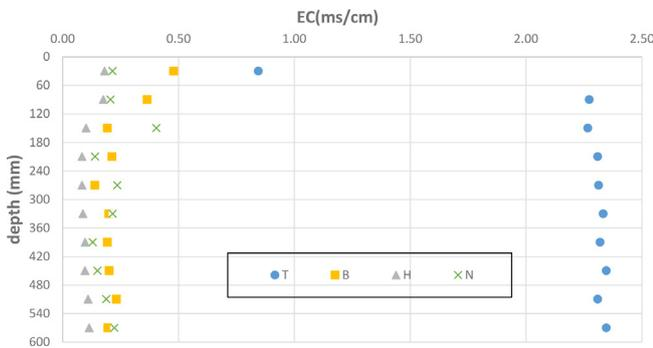
Fig. 10. The variation of the EC in the sands already used as a function of the depth of the layers.
