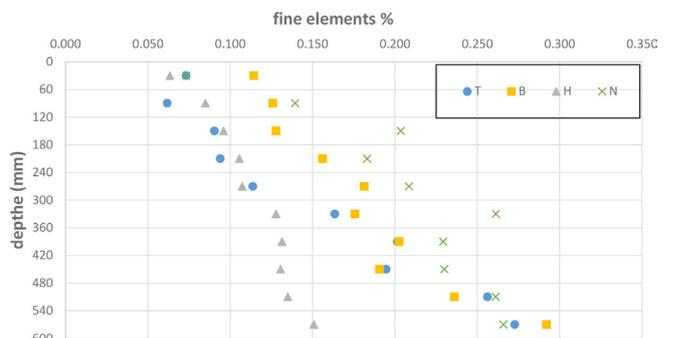
Fig. 11. The distribution of the fine particles in the sand columns.
