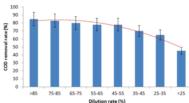
Fig. 6. Relationship between the dilution ratio and COD removal rate.
