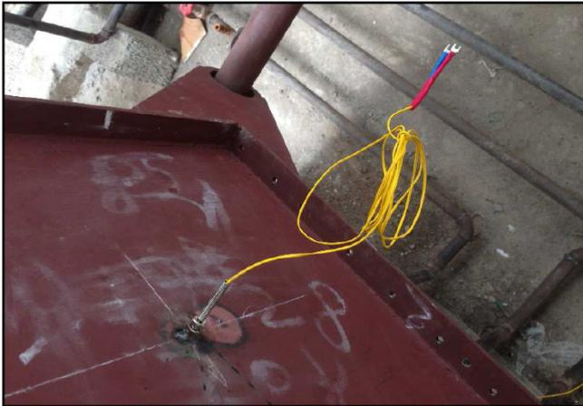
Fig. 9. k-Type thermocouple (wire type).
