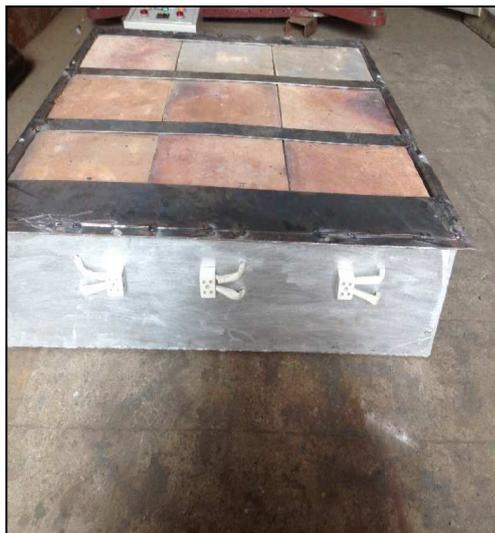
Fig. 7. Heater embedded with ceramic tiles.
