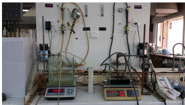
Fig. 2. FO unit with cit-MNPs as draw solution.
