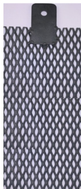
Fig. 2. Electrode used in hybrid electro-chemical reactor.
